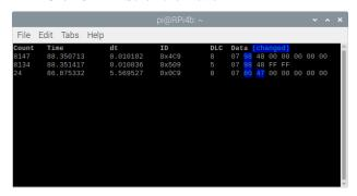
A byte in the data field is highlighted blue if the value is different from the last time the message was received.
